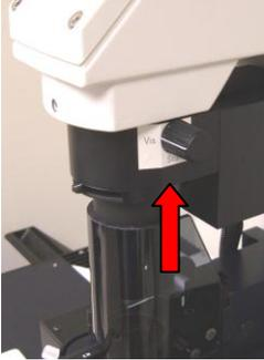
For any transmitted light observation (bright field, DIC, phase contrast), this knob should be in the **vis** position.
