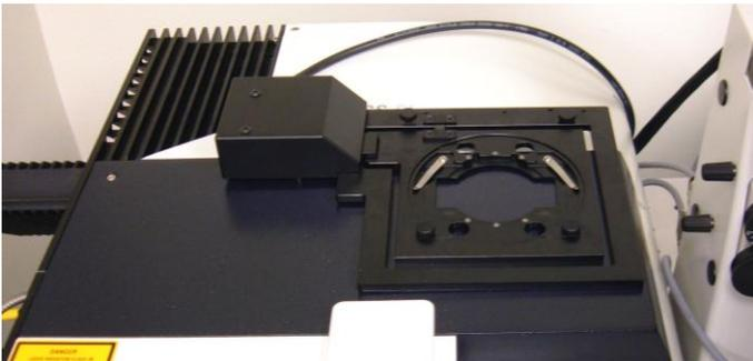
Take care not to touch condenser lens surface when removing and replacing the stages!
