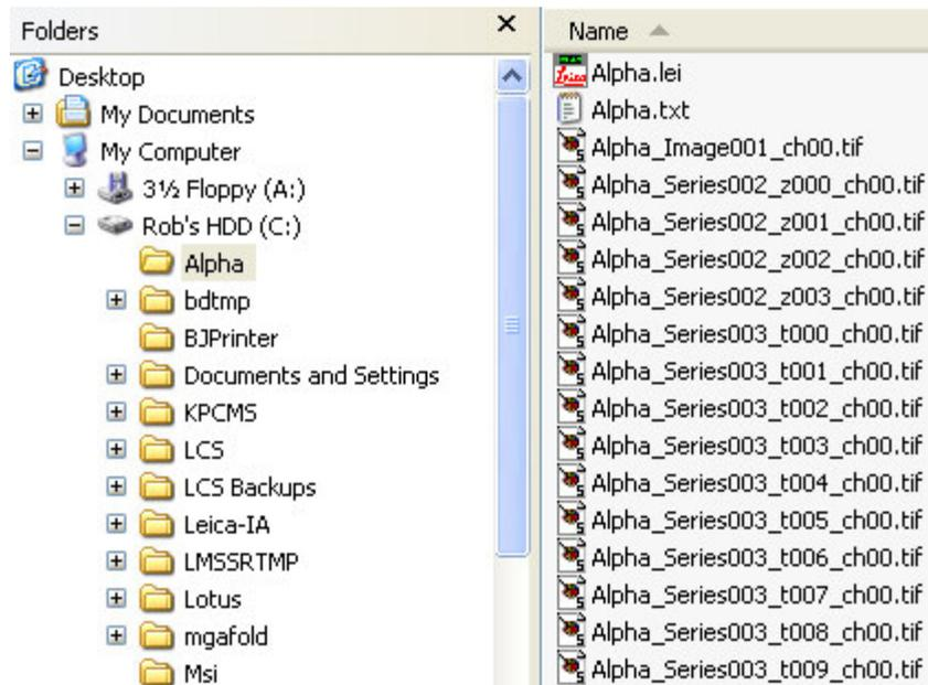
When backing up image data, the entire folder should be saved to a backup location (burned onto a CD, saved onto a network server, etc.). Note that the .lei file contains organizational information for all of the files in the Experiment folder when they were last saved in LCS. Any .tif file names that are changed or deleted outside LCS may present difficulty when reopening the Experiment.
