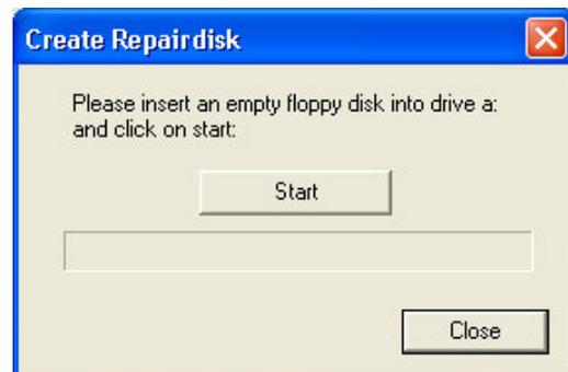
You can then press start and the program will automatically load the necessary backup information from your system onto the floppy disk. This repair disk will contain all the necessary calibration files for your system. Save this floppy disk in a safe spot. The disk may come in handy if the confocal workstation needs major repair or the operating systems needs to be rebuilt.
